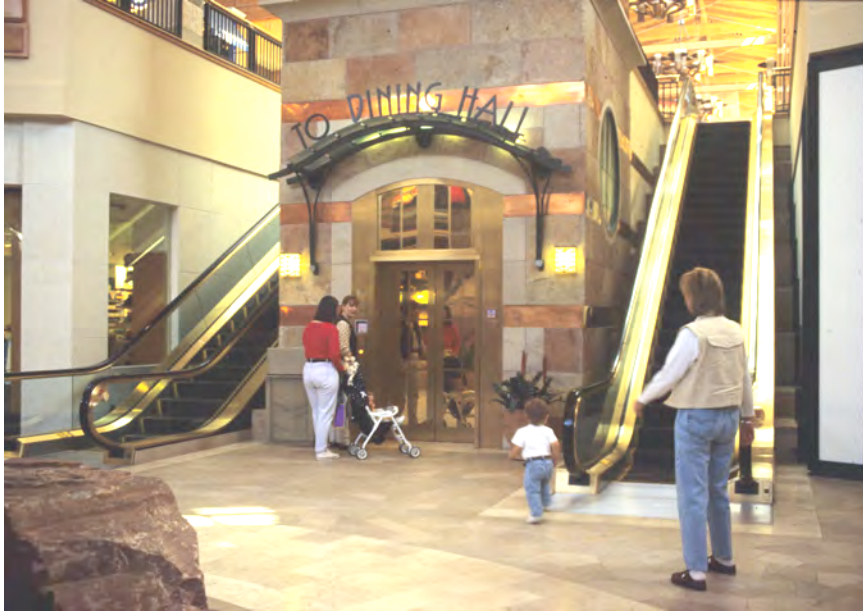
Figure 4: Locating the elevator and escalators together avoids segregating group members with different modes of mobility. Photo Credit: Center for Universal Design
